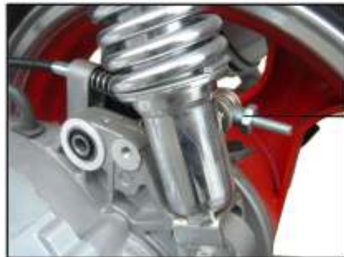
Nut of Rr brake adjusting
