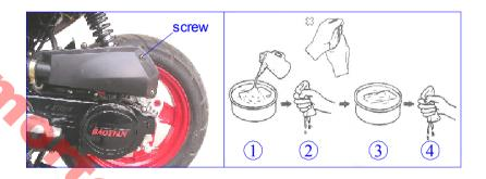
**A:** Remove 6 tightening screws of air cleaner cover. Remove air cleaner cover.
