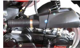
tightening screws of air cleaner cover
